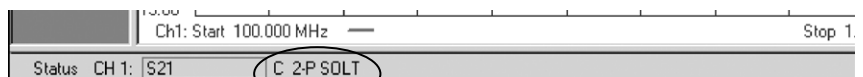
Figure 5. The MW PNA status bar provides you with valuable information, including the calibration type and status.
